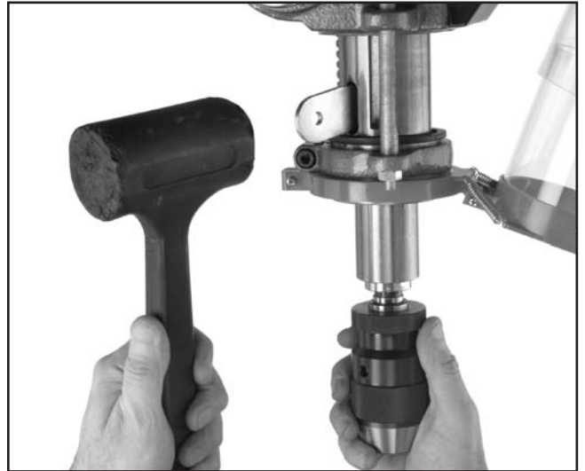
Figure 33. Using drift key to remove arbor.
